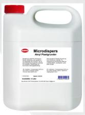
Gjøco Microdisperser is a waterborne, unpigmented primer for mineral surfaces both indoors and outdoors. The product has a very low particle size combined with low viscosity, which enables very good penetration properties on porous substrates. Used on untreated concrete, lightweight concrete, plasterboard and plastered surfaces. Binds loose particles on the surface and improves adhesion for future painting.
