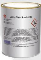
Gjøco Sinkoksidpasta contains zinc oxide intended for Herregård Linoljemaling to give the paint better properties and make the paint film more durable. Gjøco Sinkoksidpasta is especially recommended for white and light colors. It is supplied in 1 liter packaging and should be added to 9 liters of Herregård Linoljemaling. NB: Do not use in other types of paint.
