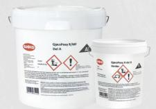
GjøcoPoxy R is a two-component, low-viscosity, solvent-free primer. It is intended for use on mineral substrates such as concrete and cement-based surfaces. It is applied to untreated substrates before further coating with epoxy or polyurethane. GjøcoPoxy R has a fast curing time and is designed for use at low temperatures down to +5 °C.
