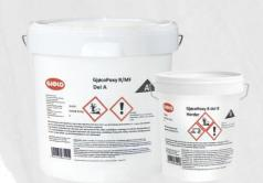
GjøcoPoxy R is a two-component, low-viscosity, solvent-free primer. GjøcoPoxy R is designed for use on mineral substrates such as concrete and cement-based surfaces. It is applied to untreated substrates before further treatment with epoxy or polyurethane. GjøcoPoxy R has a fast curing time and is intended for use at low temperatures down to +5°C.
